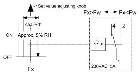
Fx = Relative humidity of the air (actual value) Fw = Humidity adjusted on the knob (set value).
