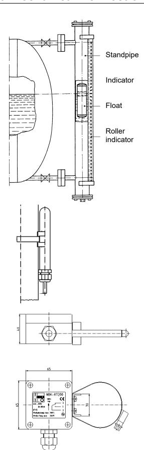
Remove bottom flange from bypass tube, and insert the cylindrical float in the NBK bypass tube with the designation "TOP" at the top. Re-position the gasket and close the bottom flange again; firmly tighten with screws. Mount and tighten the bypass tube to the vessel to be monitored with process connection and seal.
